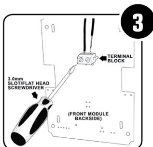
**3** Insert signal wires (2) into the terminal block, located on the backside of the front module. Secure them in place by tightening the terminal screws using a small 3.0 mm slot/flat head screwdriver (not included).
