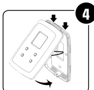
**4** Attach front module to mounted back plate, first by hooking the top of the front module to the top clips of the back plate, then by pressing the bottom of the front module until you hear a 'click'. Ensure the ventilation system operates correctly.
