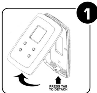
**1** Detach front module from back plate by pressing the tab (located at the bottom of the control casing).
