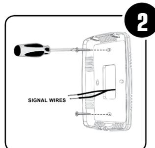
**2** Guide the signal wires (2) through the central opening of the back plate and mount this plate to either a standard electrical device box or directly to the wall using screws. If required, use wall anchors.
